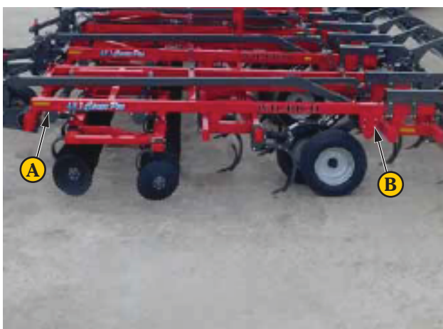
Figure 3.19 Field Operation Leveling Adjustments I
