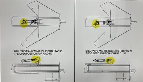
BALL VALVE AND TONGUE LATCH SHOWN IN THE OPEN POSITION FOR FOLDING
