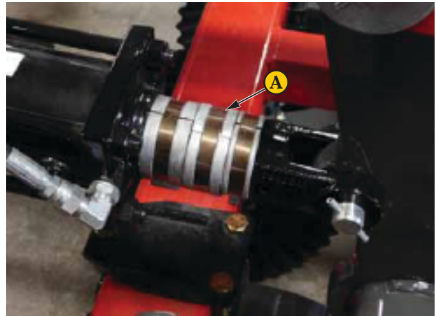
Figure 3.28 Disk Depth Setting II
