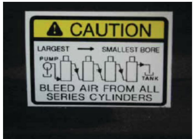
Figure 2.7 (4) Bleed Air From All Series Cylinders
