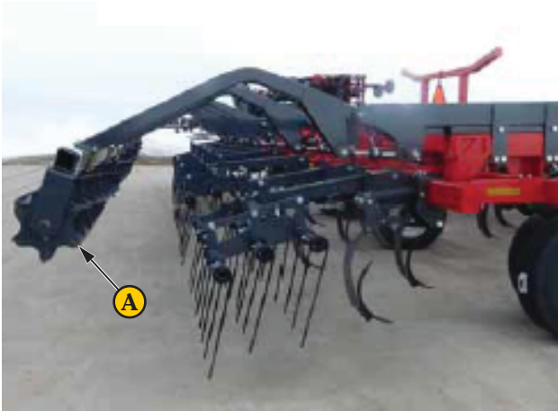
Figure 3.29 Flat Bar Rolling Basket Setting I
